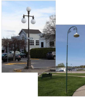
Globe Lights with 3 or 5 globes help illuminate streets and sidewalks in the Central Downtown zone and at intersections in the Downtown Waterfront zone. Shepherd's Hook Lights with Dark-Sky friendly cutoff shields illuminate the sidewalks on Bay, 3rd, North Spring and Gardner Streets.
